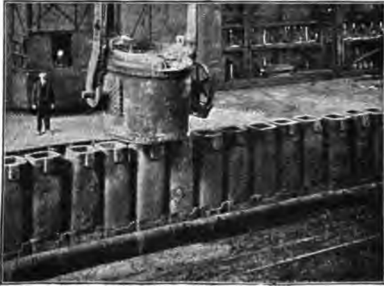
Fig. 102. The Car-casting System of F. W. Wood.
